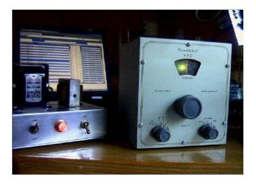
It was during this 'haywire' bench testing phase that I was able to make some power measurements and experiment with coupling a VFO into the Colpitts oscillator while using it as a buffer stage. As it turned out, the circuit worked just fine with no changes, allowing the VFO output to be plugged directly into the crystal socket with no switching required. Using the venerable Heathkit VF-1, drive levels were at the same level as
