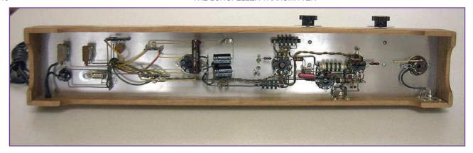
The coaxial antenna socket and key jack were brought out on the back side.
